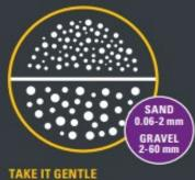
For sand and gravel you can achieve highrated state. The level of compaction depends more on grading than on moisture. Too much compaction of sand and gravel is like beating a concrete wall with a sledgehammer. It can crush the material and reduce the load bearing capacity.
