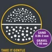
For sand and gravel you can achieve highrated state. The level of compaction depends more on grading than on moisture. Too much compaction of sand and gravel is like beating a concrete wall with a sledgehammer. It can crush the material and reduce the load bearing capacity.
