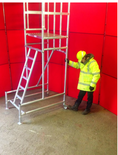
4) POSITION UNIT AND LOCK CASTORS
