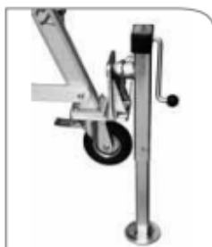
Fig.2 Jacks secured with locking pins and clips
