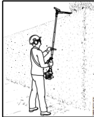
Overhead Cut (with cutter bar at an angle)
