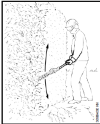
Vertical Cut (with straight cutter bar)
