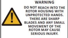
Allow machine time to clear excess chips still remaining in rotor housing before you continue feeding brushwood. Feed in a small piece of wood while watching to make sure that it comes out of the discharge. If this does not clear it, repeat the process and carefully inspect the discharge tube to find any obstruction.
