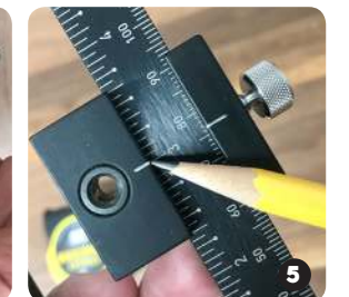
Transfer your hardware measurement to the sliding drill bushing and tighten
