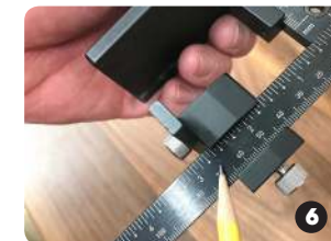
Match bottom measurement with sliding end stop and tighten.
