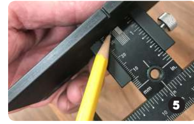
Match Large Stop to your side measurement and tighten
