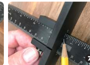
Match side measurement to Large Stop and tighten
