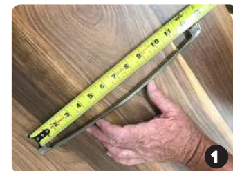
Measure hardware hole spacing
