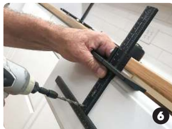
Drill hole using fixed center drill bushing
