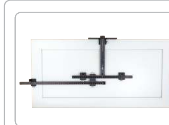
If your handle pattern interferes with double bracket move below t-square and connect the 0" ruler at the 2" mark as pictured above
