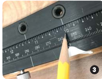
Mark selected drill bushing with tape on extension (included in TP-2312, TP-1935)
