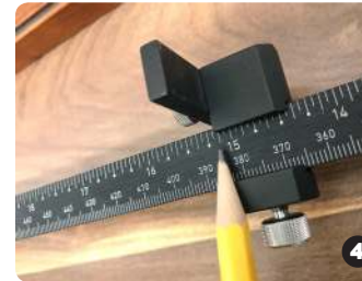
Adjust end stop at desired distance from the marked bushing
