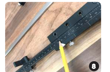
Set end stop at desired distance from center line of bushing
