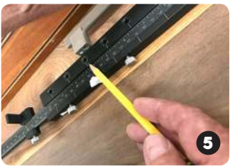
Lay the pull on the jig align with taped hole
