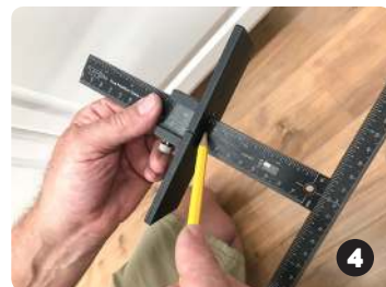
Slide Large Stop to match side measurement
