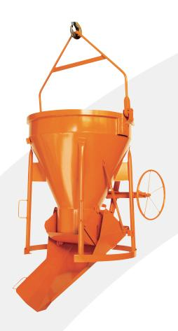
The 1020H is the ideal concrete skip for quick pouring of concrete in high volume where accuracy is not a requirement. Together with the benefit of a fold away chute which can be used to direct the pour when necessary. Available with a geared gate mechanism and a choice between fixed lifting arm and lifting chain set.
