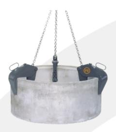
Torsionally rigid, light-weight hollow steel construction for the transportation and placement of manhole rings. The pipe tackle complies with official labour safety regulations and is equipped with a safety lock. Inadvertent slipping of the load through the claws is prevented by a spring on each clamp.
