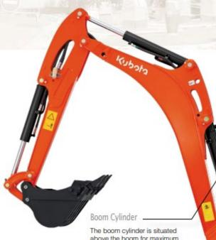
The boom cylinder is situated above the boom for maximum protection, especially during breaker or dumping operation. Movement speeds of front attachments and lifting power have been well adjusted, thanks to the boom cylinder's large-diameter rod and optimal hydraulic pressure.
